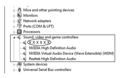
To confirm a successful installation of the video camera, navigate to Computer Properties/Device Manager/
